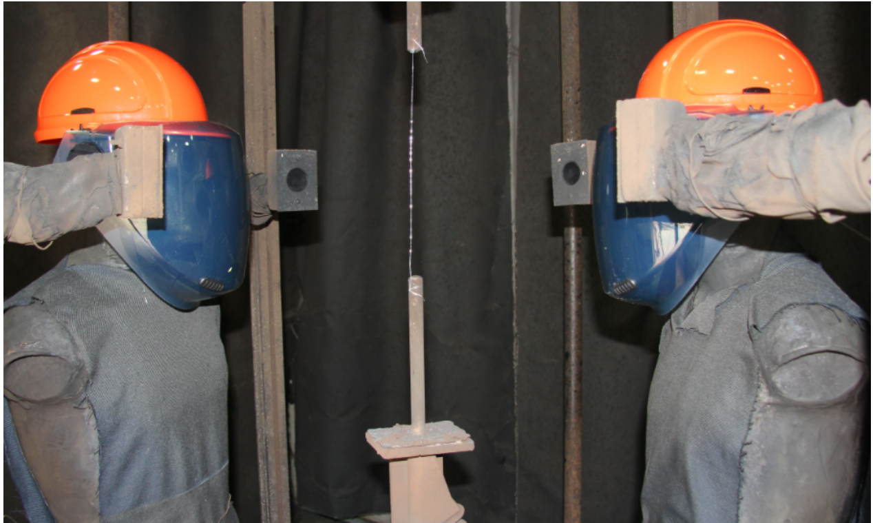
Figure 1. Faceshield before arc exposure.
