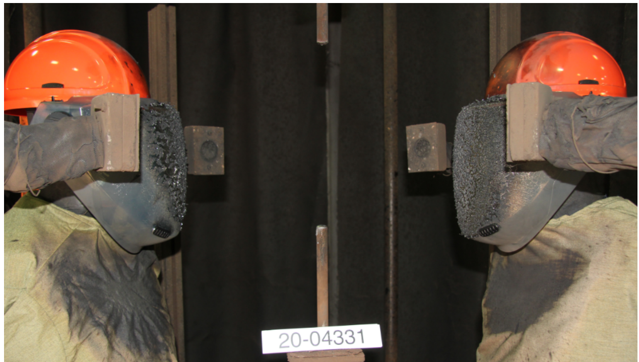
Figure 2. Faceshield after arc exposure at 18.6 -19.4 cal/cm 2 .
